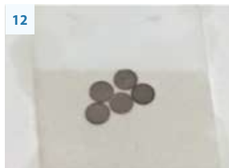
TEM grids covered with carbon floated from mica (5nm C deposited in vacuum of 7E-07mbar)
