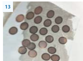
TEM grids covered with 10nm C prepared in vacuum 4 E-05 mbar, visible cracks in carbon layers
