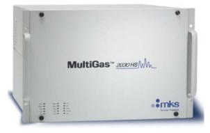
The MultiGas<sup>™</sup> 2030HS gas analyser is composed of a high-speed 0.5 cm-1 process-hardened FTIR spectrometer. This spectrometer incorporates a patented 5.11 m high-optical-throughput 200 ml gas-sampling cell capable of 100 SLPM flow rate without backpressure or noise that would degrade the quantitative measurement. The analyser also incorporates a high sensitivity liquid nitrogen cooled MCT-detector.
